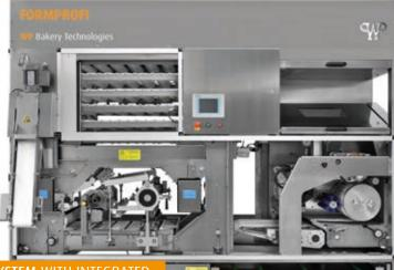
**COMPACT FORM BAKING SYSTEM** WITH INTEGRATED DRUM MOULDER FOR THE PRODUCTION OF
