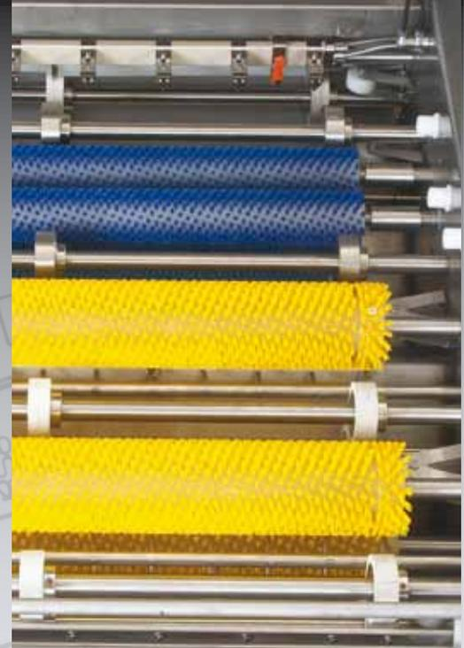
The system can be used for large Capacity of 800 - 1000 trays per hour. The trays are taken through the system and cleaned with the baking side up, which means that the trays are ready to be used right away without any need to turn them over.
