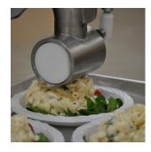
The PRO 1000i Food Service depositor is designed for ultimate sanitation requirements in Food Service areas to work over production lines and conveyors to increase efficiency. It can be used for quick and clean depositing of all flowable products including fillings, spreads, salads, soups and sauces, condiments and much more. Of course this industrial depositor can be fitted with a wide variety of more than 100 Unifiller attachments.
