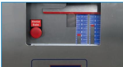
The number of the blades determines the number of layers to be sliced (e. g. four blades = max. five layers).
