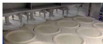
Various product shapes can be cut by the same cutting module and cutting change-over tools.
