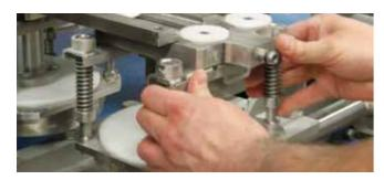
Efficient, error free operation and tool change-over is realized by applying Unique Fit Tooling. Because of the lightweight and more compact tooling, handling and detaching the tools is as easy as possible and can be done by one person.
