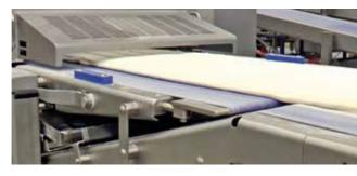
Elimination of falling heights: by minimizing the transportation height throughout the production line, it results in a stable and relax dough sheet.
