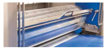
Wear resistant roller scrapers to keep the rollers of the reduction stations as clean as possible.
