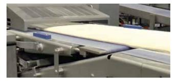
Elimination of falling heights: by minimizing the transportation height throughout the production line, it results in a stable and relaxed dough sheet.
