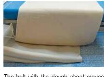
The belt with the dough sheet moves back and forth above the next conveying belt. This is an asymmetric lamination system suitable for soft dough with no restrictions regarding laminating width.
