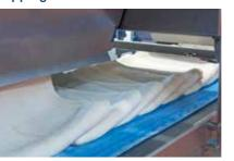
The dough sheet runs vertically between a guiding system that moves back and forth. This symmetric lamination method is unsuitable for soft dough and has a maximum lamination width of 600 mm.
