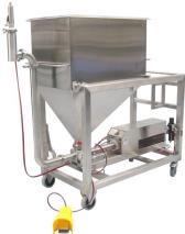
Example picture; Pro 2000i LL equipped with 270 litres rectangular hopper
