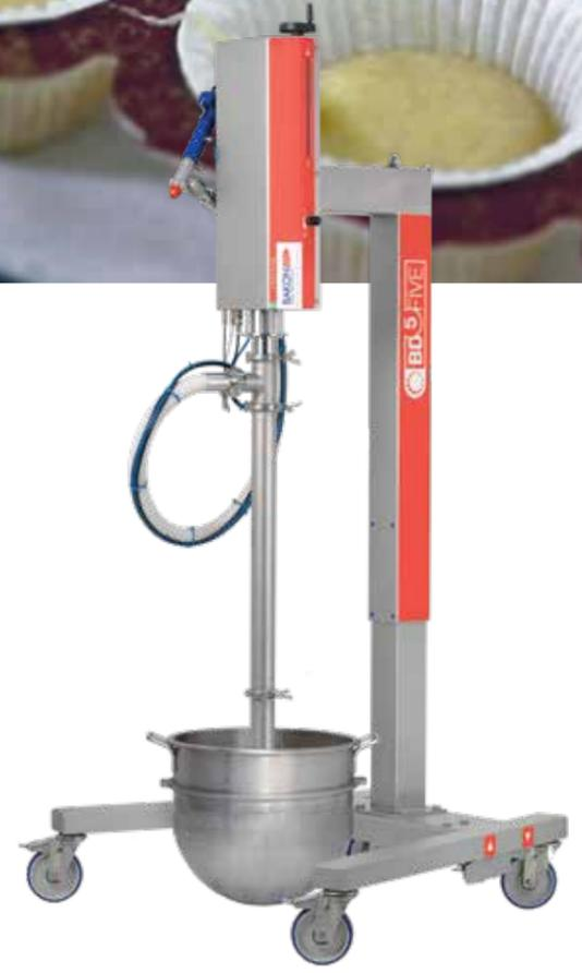
The BD5 is a high-performance pump and depositing machine that deposits your products with great accuracy. This BD Depositor is easy to handle and is easily movable on swivel casters.
